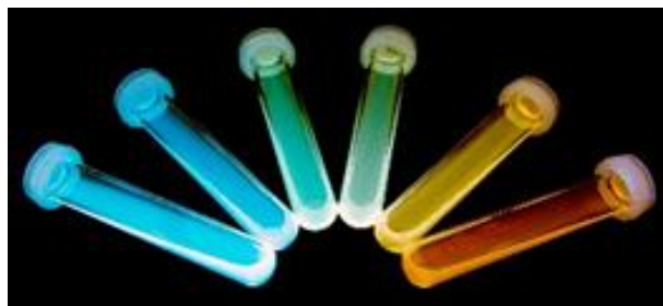
Figure 1: The fluorescence of the carbon dots can be tuned from the blue to the far red/near-infrared regions of the spectrum.
